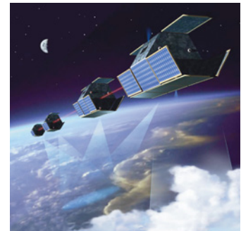
ONERA Romulus concept: Earth observation with radar satellites in formation, to detect surface motion
