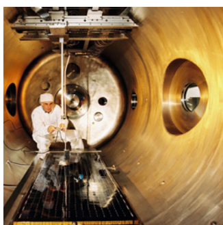
JONAS plasma chamber, enabling the production of an ionospheric-like plasma
