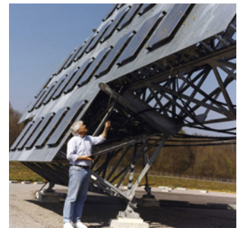
Transmitting antenna of the Graves space surveillance demonstrator, now operated by the French Air Force
