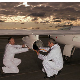
Optronic sensor integration into the pod of ONERA's Busard motorglider
