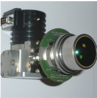
Wide-field curved-sensor infrared camera demonstrator (Temoin DGA project with Sofradir)
