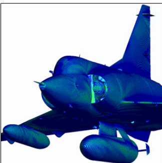
Numerical simulation of surface currents on a Mirage III subjected to an EM wave
