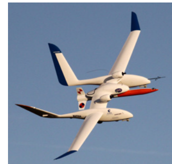
Eole: automated and reusable aircraft demonstrator for placing small satellites in orbit
