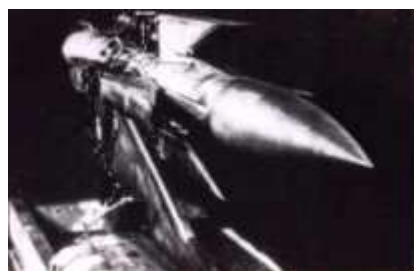
Model for S4 wind-tunnel testing
