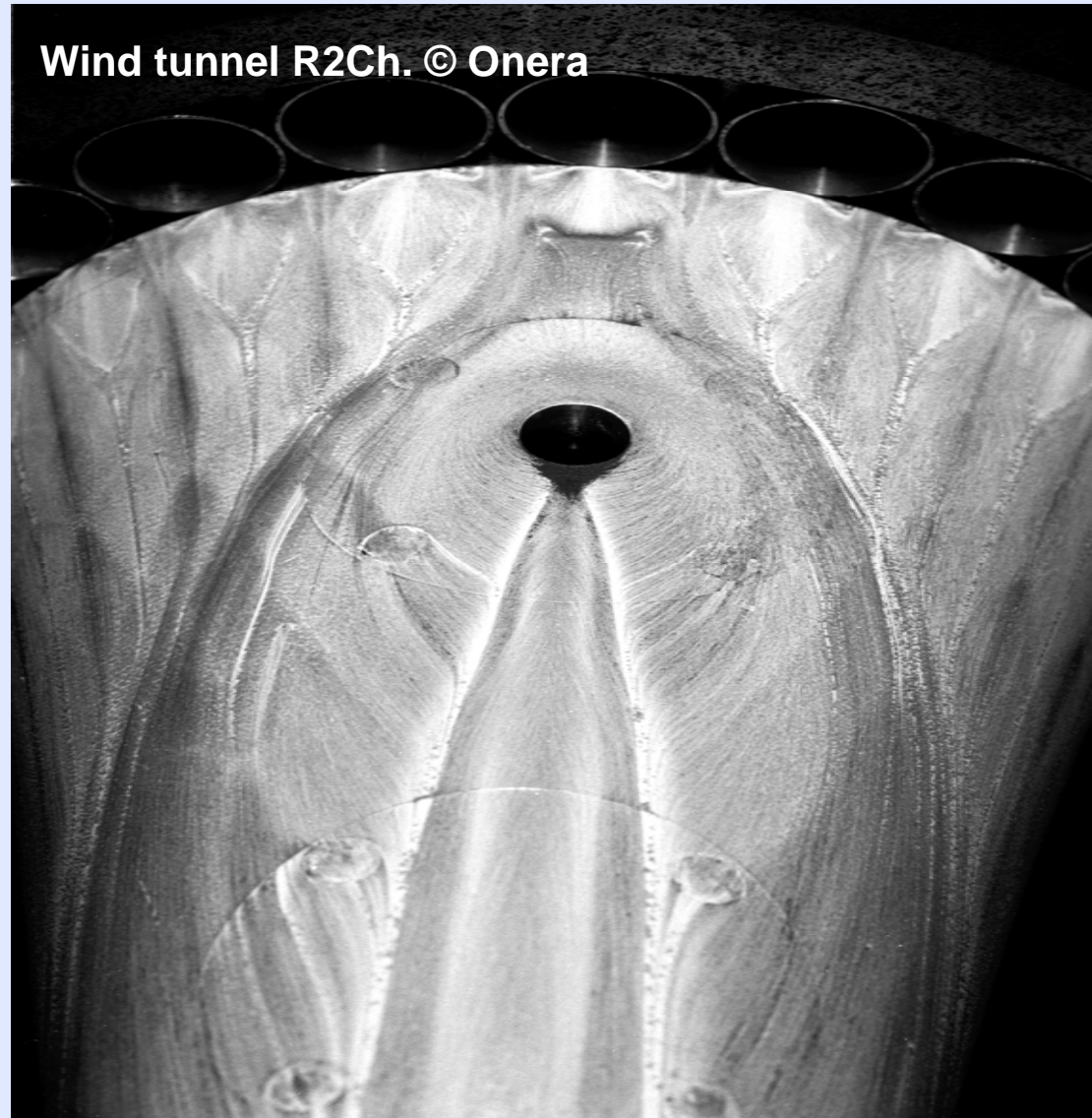
Surface flow visualisation. Lateral jet exit region
