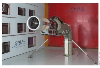
Air Intake tests: head-wind or cross-wind. Ground effect simulation. Reynolds number close to full scale. Air intake mass flow up to 75 kg/s.
