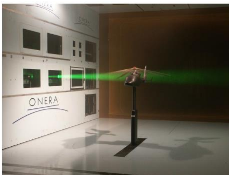
Full helicopter model test in F1
