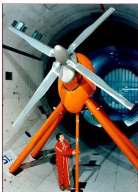
Isolated rotor model test in SIMA
