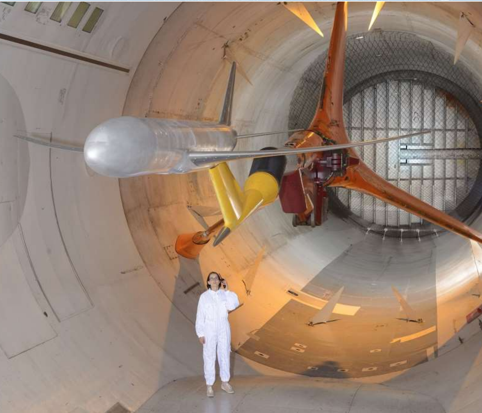
ONERA Large Reference Model in the transonic wind tunnel S1MA – Modane, France
