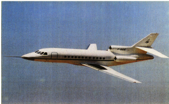
Figure 4 : Falcon 900 flight test with two HLF inboard wings
