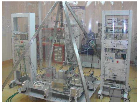
Figure 8: Pendulum test bench for gradiometric pair functional testing.
