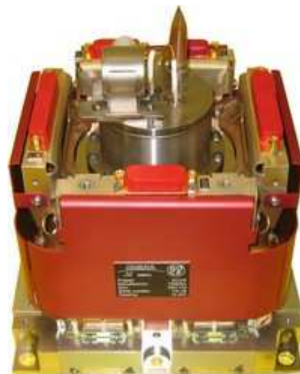
Figure 5: ASH-05 before delivery to Thales Alenia Space Gradiometer Team. On the top of the ASH, there is the ionic pump used during functional test on ground and the getter housing .
