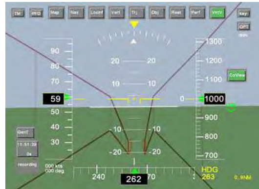
Figure 5: Approach phase with an identification mark of the VFR decision height at 200 ft AGL
