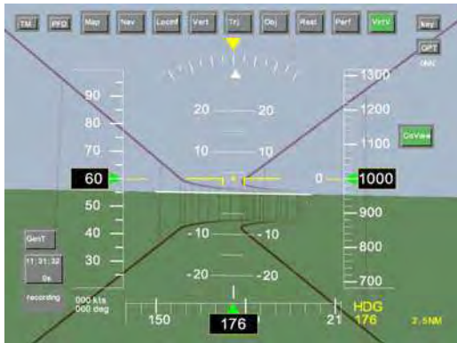
Figure 4: Enroute flight with tunnel display
