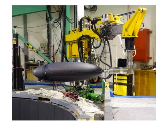
**Bench** for characterization (aerodynamic and acoustic) of **Propeller** of large size: diameter up to 2 m, rotation up to 1500 rpm, torque 160 N.m associated with **Anechoic chamber**, compatible also with BMS support.
