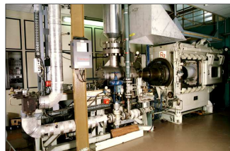
Veine d'essai L=1,570m, l=1,055m, h=1,8m
