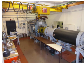
Veine d'essai L=1,570m, l=1,055m, h=1,8m
