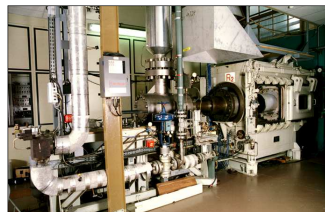
Veine d'essai L=1,570m, l=1,055m, h=1,8m
