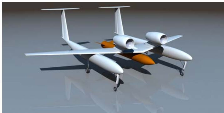
A possible vehicle architecture for the future ALTAIR air-launch system
