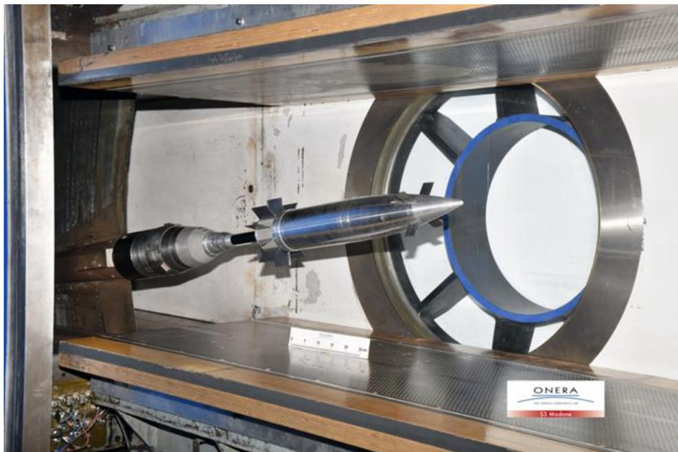
The first campaign focused on the guided part of the flight, from the opening of the CAS (Control Actuation System - set of control surfaces), a device enabling trajectory control, until target arrival (see diagram). It made it possible to refine the digital models and test different ammunition configurations throughout the planned flight range.
