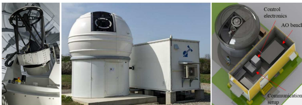
Figure 1 : Key components of the FEELINGS ground station. Left : 600 mm telescope, center : dome and shelter, right : control electronics, AO bench and communication setup location in the shelter.
