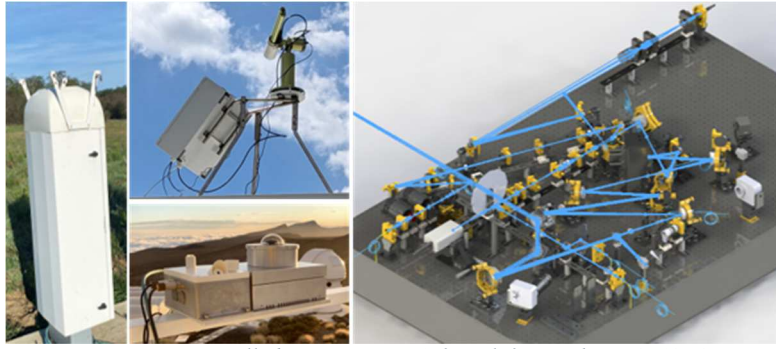
Figure 2 : Atmospheric monitoring equipment installed on FEELINGS, from left to right : VAISALA's CL51 ceilometer, CIMEL CE318 Sun-Sky-Lunar spectral photometer, Miratlas Integrated Sky Monitor including a visible all-sky camera, ONERA's AO bench.
