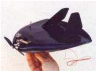
Fig. 2 : Voilure fixe Black widow, Aerovironment, USA
