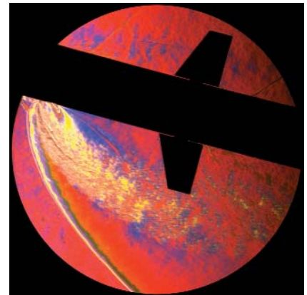
Coloured schlieren methode: transversal jet interaction on a control surface (M902140).
