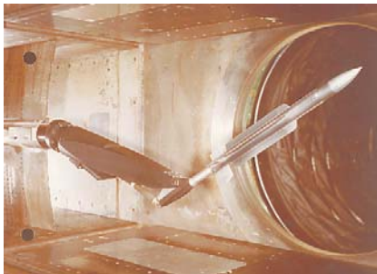
Set-up for high angle of attack missile test (C12140).
